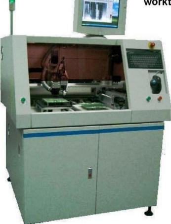
With two independent work tables it increases production efficiency and throughput, by allowing the loading and unloading of PCB panels from one worktable while the PCB panel on the other worktable is being depaneled.
